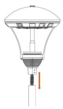
2. Using a hex key, tighten the six set screws to secure the fixture to the pole.
